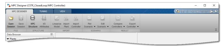
Using **MPC Designer**, you can define the MPC structure by linearizing the Simulink model. After you define the initial MPC structure, you can also linearize the model at different operating points and import the linearized plants.
